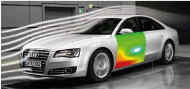
**Trim Engineering** – Trim selection is a critical design function in the automotive industry. The challenge of optimizing weight against cost to meet challenging interior noise targets can cause delays and cost overruns in the design cycle. With VA One, models can be created for trim optimization that are deployed as part of a collaborative effort to identify the right configuration and the right cost.
